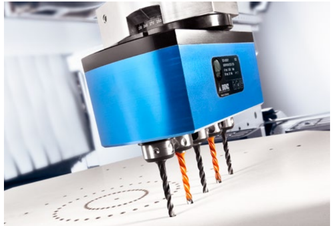
Drill rows in acoustic boards
