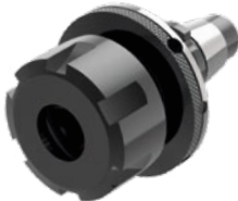
Collet chuck holder with externally located clamping nut per DIN6499 Clamping range ER 25 Ø2-Ø16 ER 32 Ø2-Ø20
