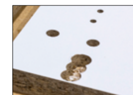
2 MULTI V3 CABINEO Drilling of pockets for Cabineo connectors in one step
