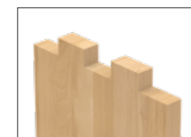
2 MOULDER Milling of finger joints
