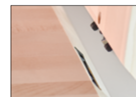
2 FLEX D Milling of profile slots for inserting the connector (e.g. Clamex connector)
