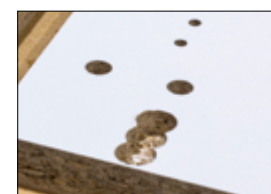
3 MULTI V3 CABINEO Drilling of pockets for Cabineo connectors in one step
