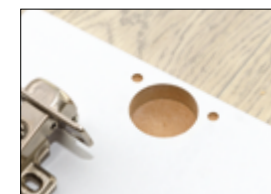
3 MULTI V3 Drilling of holes for concealed hinges
