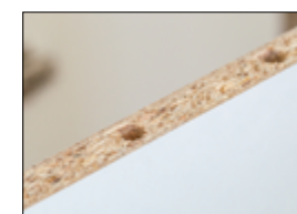
1 MULTI H3 NESTING Drilling dowel holes in corpus elements with nesting machine
