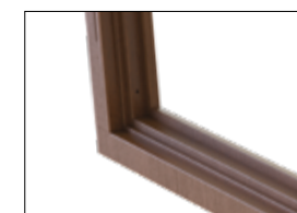
2 TRUCOLO Milling of profiles with profile milling heads
