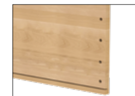
4 MULTI V5 Drilling of row holes for shelves
