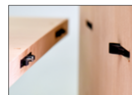
1 DUO Drilling and milling of profile slots and grooves
