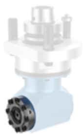
Centering Ø40 (TK Ø52 - 8x M5) /collet chuck holder ER25A per DIN6499 with internally located clamping nut
