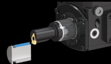
External machining of a workpiece with a broaching unit
