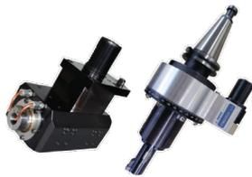
The BENZ LinA broaching system changes the rotary motion of the live tool turret into a linear motion for broach and spline machining on turning centers. The BENZ LinS broaching tool system is a one-of-a-kind system that enables programmers to broach splines, torx, hex and keyways on their machining centers.
